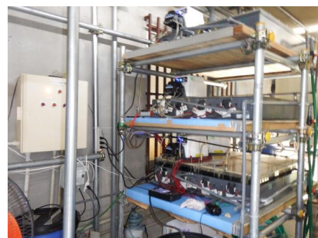
Prototype MFC at distillery operating continuously since 2013
